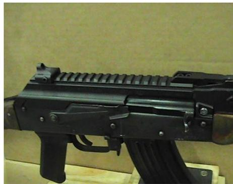
**4)** Adjust length of Dog Leg™ cover to fit weapon. Cover should be extended as far back as possible. After length adjustment re-install leaf sight spring.
