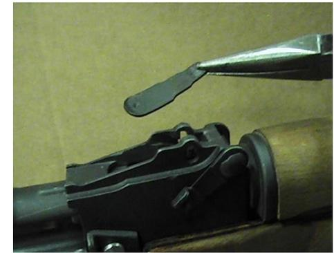
**2)** Remove leaf sight spring and set aside for installation later. Remove dust cover and recoil spring assembly.
